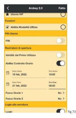
**Time Slots:** They allow a more precise control of the restrictions, within the enabling period. It is possible to indicate on which days of the week and for which time slots the restriction is active.
