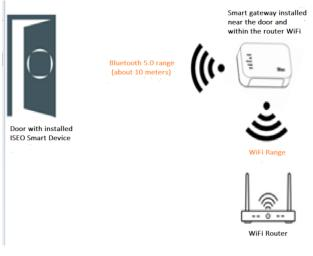
Through the Gateway Device, the inputs and door opening can be managed from anywhere in the world without being close to the door via a cloud service managed by ISEO.
