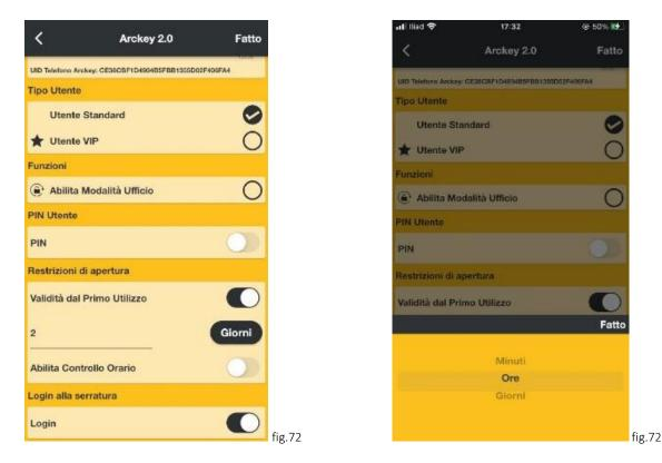
Enable time control: It allows assigning a time duration for the validity for a user (from a date to another one).
