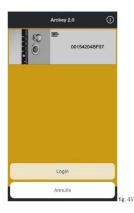
Security can be increased by adding a user PIN to the login function (see p.15). In this case, the PIN is required to authorize the access.
