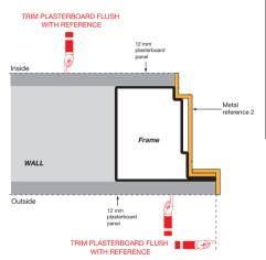
Check the width measure paying attention to check it at least on 3 points (on the top, on the bottom and in the center).
